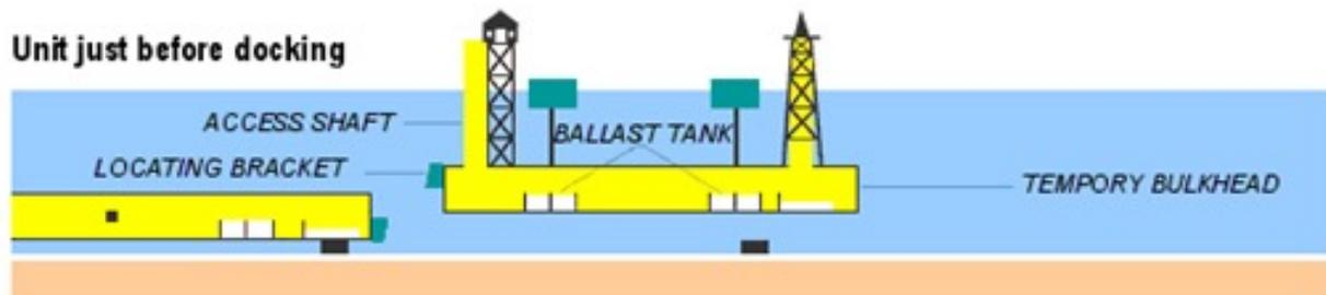
Tunnel ballasted and backfilled
